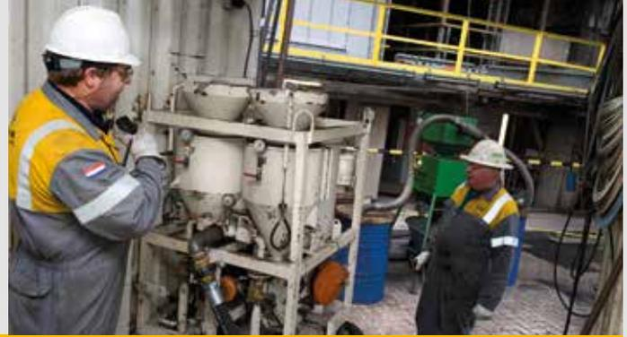
For systems where the use of water for cleaning tubes is prohibited or limited to a minimum, (Mini)Sandjet® cleaning is a safe, fast and effective option. The technique is based on a cleaning agent, shot or grit that is injected with high velocity dry nitrogen or air through the furnace tubes or pipeline system. Sandjetting is the best cleaning solution for VCM furnaces, oxygen pipelines and heat exchangers.
