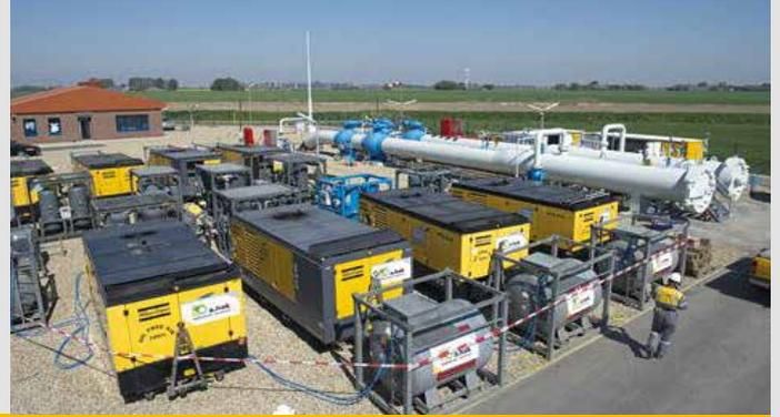
Prior to commissioning and start-up, it can be essential to carry out a drying procedure to thoroughly remove water and moisture from the system. This procedure will help to maintain the purity of the product to be transported through the system, minimize corrosion (growth) and optimize efficiency and safety.
